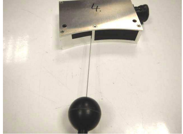
Picture 2 Sensor head MHP XXX specimen with rigid steel wire (Ø 1 mm, 1 N) during contact protection test IP6X
