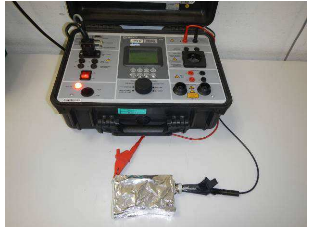
Picture 8 Sensor head MHAP XXX specimen with portable compact tester insulation test after the water immersion test IPX7
