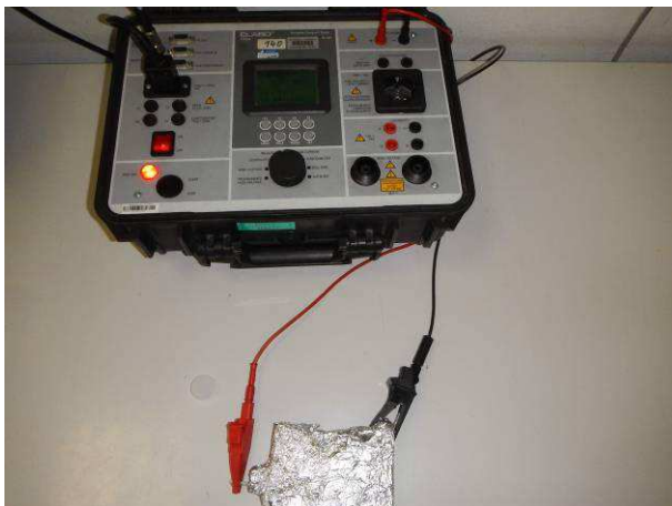
Picture 11 Sensor head MHAP XXX specimen with portable compact tester insulation test after the water jet test IPX6
