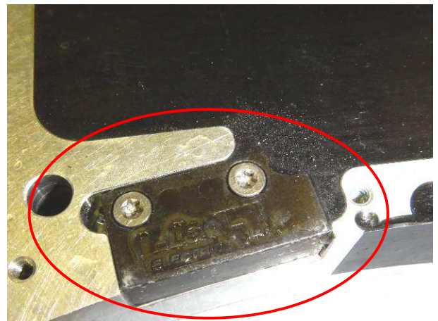
Picture 12 Sensor head MHAP XXX traces of water on the sealing compound inside after the protection tests IP67 and IPX6
