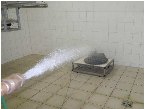
Picture 9 Sensor head MHAP XXX on the turn table with water from the spray nozzle during the water jet test IPX6
