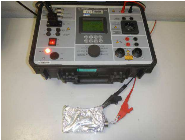
Picture 3 Sensor head MHP XXX specimen with portable compact tester insulation test before immersion substitute test IP6X
