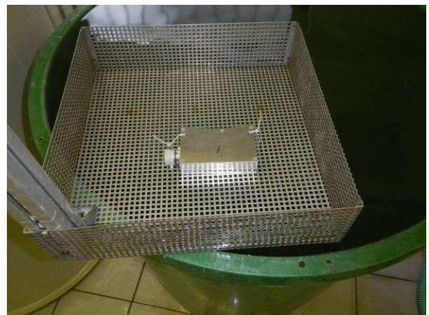
Picture 5 Sensor head MHP XXX specimen with portable compact tester insulation test after the immersion substitute test IP6X before the immersion substitute test IP6X
