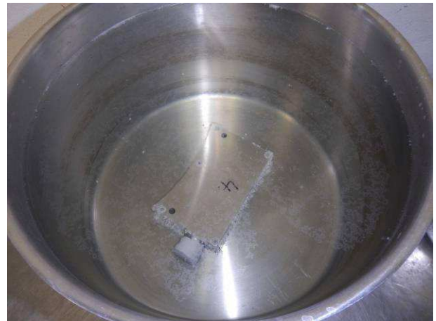
Picture 4 Sensor head MHP XXX specimen in the dipping basin 200 mm during the immersion substitute test IP6X
