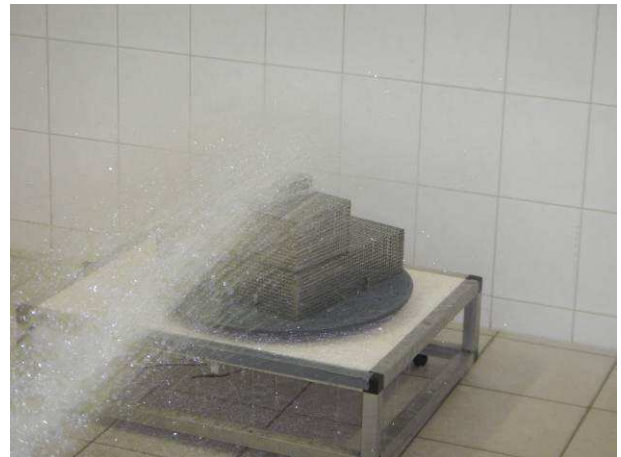
Picture 10 Sensor head MHAP XXX on the turn table with water from the spray nozzle during the water jet test IPX6
