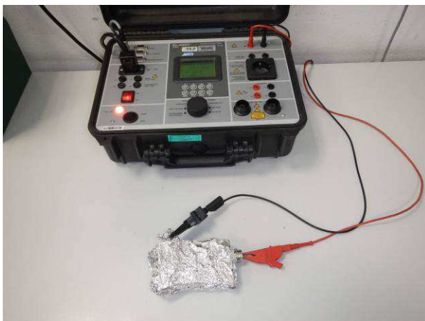
Picture 5 Sensor head MHP XXX specimen with portable compact tester insulation test after the immersion substitute test IP6X before the immersion substitute test IP6X
