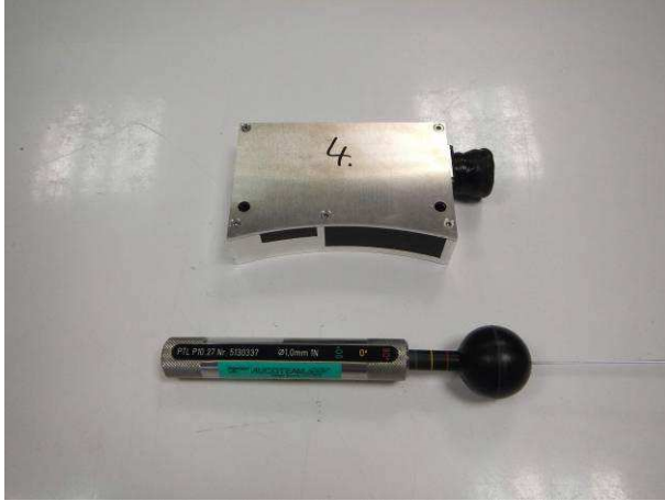
Picture 1 Sensor head MHP XXX specimen with rigid steel wire (Ø 1 mm, 1 N) during contact protection test IP6X
